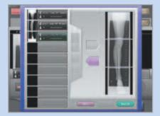
**Xpress Digital Image Stitching** Important for applications such as Scoliosis and other long length bone studies, this option enables the acquisition of multiple images from a single exposure and allows electronic "stitching" to form a single image. The image can then be used in applications where bone measurements are made.
